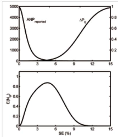
Figure 3. The expected number of unacceptable results —  $E(N_U) = \Delta P_E \times ANP_{reported}$ ; for this case,  $E(N_U)$  reaches its maximum at 4.7% systematic error.
